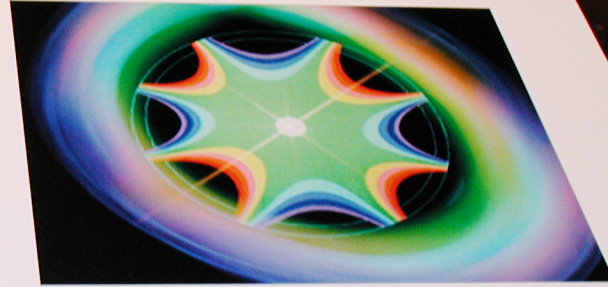
March 1987 Brockhaven National Laboratory The magnetic field surrounding a superconducting magnet is represented here in false color that varies with the strength of the field. This happens to be the field surrounding one of the 1,743 magnets that surround the Brookhaven heavy ion Collider, a particle accelerator at Brookhaven National Laboratory. The magnetic fields push and pull particles around the 3.4-mile circumference ring.
